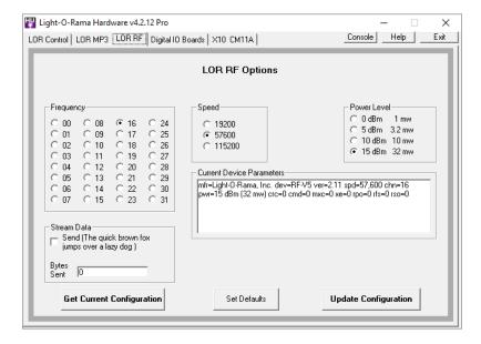
The transceiver must be the only transceiver unit connected to the PC. The transceiver must be connected to the PC with an LOR USB485B adapter unless there is also a LOR controller daisy chained which will supply accessory power.
