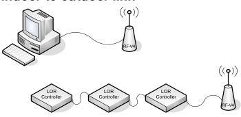
The Easy Light Linkers are used to transfer data from the indoor PC directing the show to the outdoor controllers. Aside from the obvious advantage of not requiring a hole in the house for the wire, it also completely isolates the PC from the outside world. Even if a controller is knocked over and allowed to fill with water, there is no possibility of AC voltage getting into the cable to the PC.
