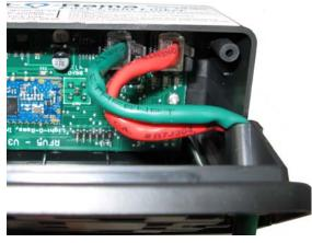
If you want to place the ELL on a flat surface, the wire exit tab on the case can be snapped off.
