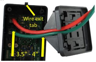
Pull the wires into a small loop and snap the base plate into the RF-V5 as shown below:
