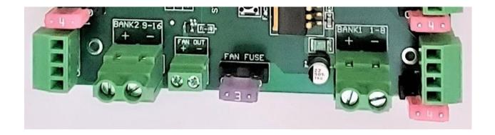
The board can run on any voltage between 5VDC - 30VDC. The voltage you use will be dependent on the type of pixel in use. Power must be supplied from a stable DC source/power supply. The maximum rating of the board is 64A, 32A per bank, 4A per pixel port. Each port is protected by a 4A (pink) blade type fast-blow fuse.
