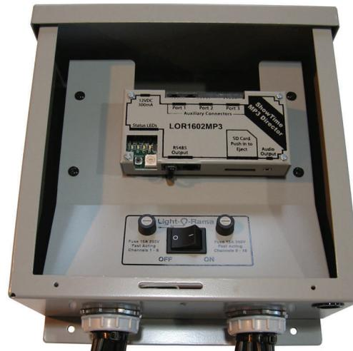
Cover removed showing the DC-MP3 daughter card installed in an LOR-1602W Lighting Controller. Picture below shows covered controller with cables for power and lights..
