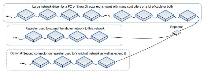
Note that the last controller on the main network is connected to the single jack side of the Repeater and the extended network is connected to the double jack side. If Y'ing is not required, then the Repeater could be inserted the other way.
