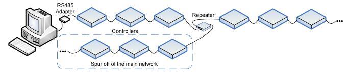
Note that the Repeater has the two jack side inserted into the main network daisy chain style and the spur network is cabled to the single jack side. You can insert multiple Repeaters in this fashion to create a number of spur networks.
