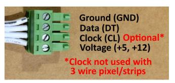
Same connector used for Light-O-Rama PixCon16, Pixie16, Pixie8 and Pixie4 pixel controllers.
