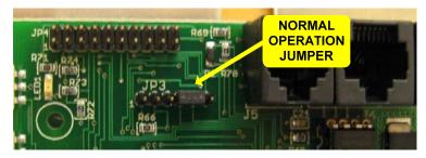
To reset the controller, power it off, move this jumper to pins 5 & 6 (one pin right) and power the controller on. The status LED will fast blink during reset. Once you see this, power the board off and move the jumper back to pins 4 & 5.
