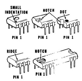
Before installing an IC, either directly into the circuit board or into a socket, you must straighten the pins. Examine the IC carefully, making sure that the pins are straight and bow outward slightly as show by the picture to the right.
