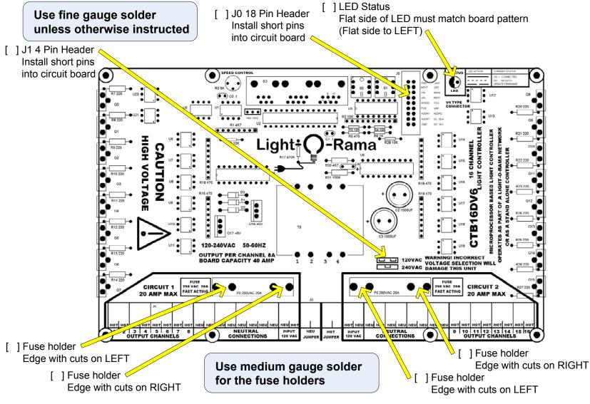
**Note:** The four fuse holder components have and 'outside' and and 'inside' edge. The 'outside' edge has small cuts to prevent the fuse from sliding out of the holder. Use a 40 watt soldering iron for these components. Make sure you completely fill the fuse holders' circular solder pads with solder.
