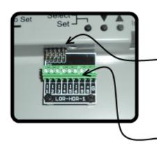
Input header plugs into the black, 10 pin connector
