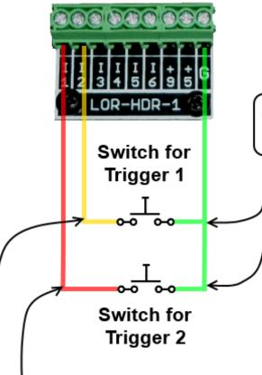
Connect one side of each switch to G (ground)
