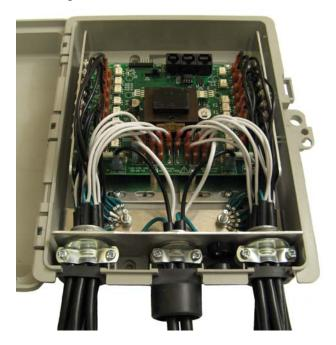
14. This completes the assembly of your controller. (Note that this picture shows the fuse covers – these were a late addition designed to protect the wires passing over the fuses.) You are ready to configure it for testing.
