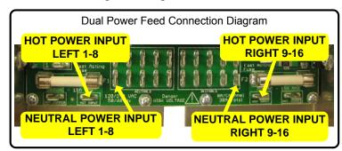
The following picture is just to illustrate the connections for the dual power feed, do not connect the wires or mount the bracket yet.
