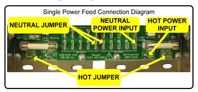
Note that in this arrangement only the right fuse is used and carries the current for both the left and right banks of channels. The picture on the next page is just to illustrate the connections for a single power feed, do not connect the wires or mount the bracket yet.
