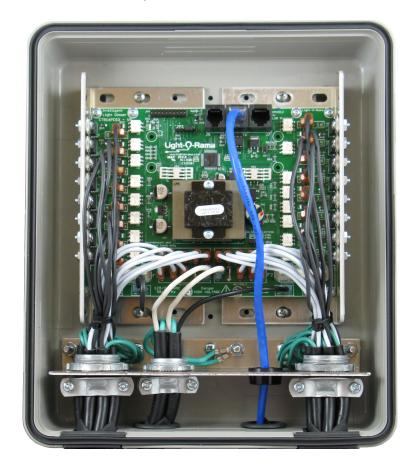
This picture shows the AC neutrals wired to the center of the neutral blocks rather than the ends as in the old manual. Either way is fine. Install the large edge gasket with the U shaped channel facing outward.
