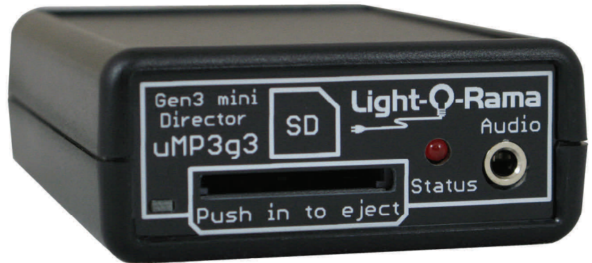
uMP3g3 module shown 2 5/8" w x 1 1/8" h x 3 3/4" d
