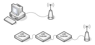
The Easy Light Linkers are used to transfer data from the indoor PC directing the show to the outdoor controllers. Aside from the obvious advantage of not requiring a hole in the house for the wire, it also completely isolates the PC from the outside world. Even if a controller is knocked over and allowed to fill with water, there is no possibility of AC voltage getting into the cable to the PC.
