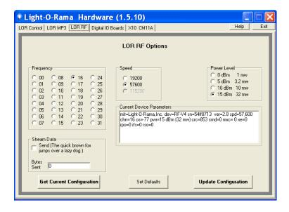
The transceiver must be the only transceiver unit connected to the PC. The transceiver must be connected to the PC with an LOR USB485B adapter unless there is also a 16 channel controller daisy chained.
